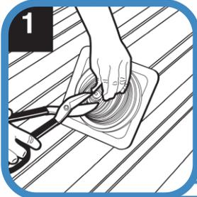
Select an appropriate Master Flash® Standard with a pipe range that goes below and beyond fitting. If necessary, use the lines clearly shown on the flashing to trim an opening 10 - 20% smaller than pipe diameter. For the steep roof slopes or higher corrugation of the profile, bigger size of Master Flash® should be chosen.
