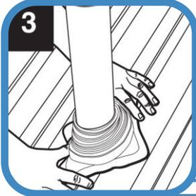
Press Master Flash® down, bending it to conform to roof profile or irregularities. A blunt tool will help to form flashing to tight roof angles.
