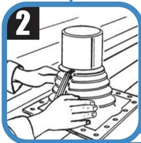
**2** Wrap Master Flash® Retrofit around the pipe. Press the flashing down, bending it to conform to roof profile or irregularities. A blunt tool will help to form flashing to tight roof angles.
