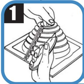
**1** Select an appropriate Master Flash® Standard Retrofit with a pipe range that goes below and beyond fitting. If necessary, follow the lines clearly shown on the flashing and create an opening 10-20% smaller than pipe diameter. For the steep roof slopes or higher corrugation of the profile, bigger size of Master Flash® should be chosen.
