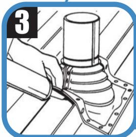
**3** Apply sealant between the base roof and at the top of the flange.
