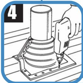
**4** Fix the flashing using self-drilling screws. Spacing between fasteners must not exceed 38mm (1.5").
