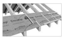
3. Nail the counter-battens in such a way as to cover the points of the membrane punctured with staples or roofing nails. In order to seal the membrane, it is recommended (in case of roofs with pitches below 20° it is required) to apply sealing tape (e.g. Corotop Pur) on the pressure side of the membrane before installing
